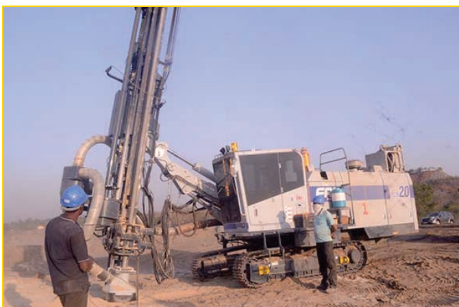
Furukawa make heavy duty wagon drill machine
